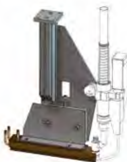
Dia. D - 51 TIG - Torch Mount with Purging (s. Chapter F)
